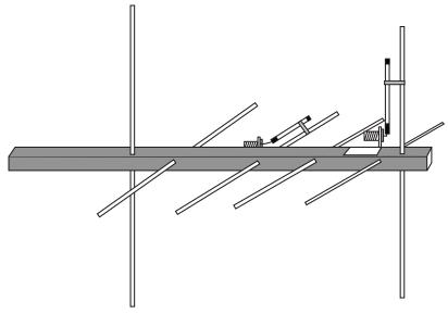
Elements mounting are through hole. Elements are fastened with a screw drilled at the center of the boom screw is chosen as to touch the wall of the boom but does not penetrate the opposite side for cleaner look for more hold you may drilled through the boom and use a screw that protrudes a bit to the opposite side and put a nut on it. Antenna feed point is dual connected by a 1/4λ phasing harness 75ohms optimize for the VHF center frequency 145 Mhz
