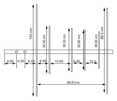
Measurements are all in centimeters. You may adjust the handle measurements depending on your preference for comportable hold.
